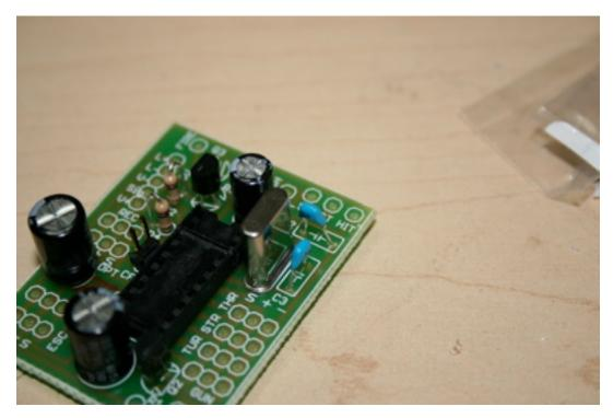
Solder in the 20mhz crystal at Q1, and the 20pf capacitors at C2 and C3 (no polarity to match).
