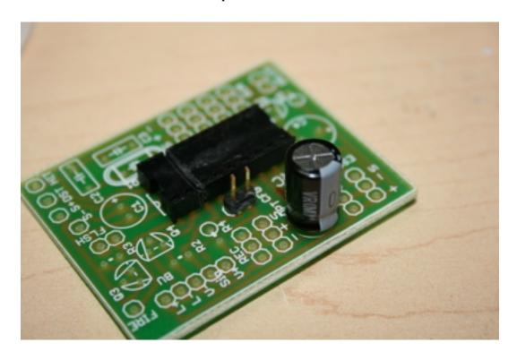
Solder in the 2 pin jumper header at "CFG" and a 470uF capacitor at C5. Make sure the capacitor matches the polarity on the silkscreen.
