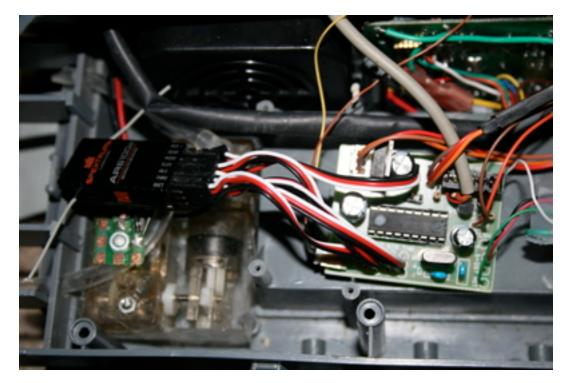
Install the PIC chip in the socket, making sure you match the notch in the chip with the notch on the board/socket. Connect the Heng Long jumper cable to the "ESC" socket.
