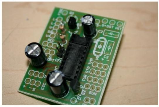
Solder in two BS170 FETs, one at Q2 and the other at Q4, being careful to match orientation with the silkscreen.
