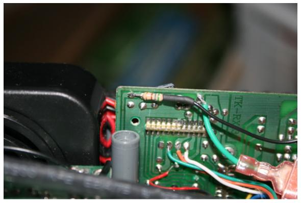
If you wish to connect the sound chip to the Heng Long sound system, connect the long wire from the capacitor to this point on the Heng Long board. You may optionally use a 560 ohm resistor (green, blue, brown) as shown to provide a more matched sound, but with less "impact". Insulate the sound card and connections with electrical tape to prevent shorting (but leave the buttons un-pressed).
