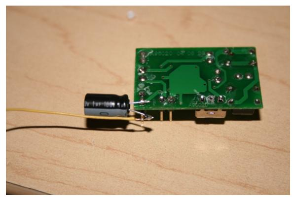
If you're connecting the output to the Heng Long sound system, solder the positive pole of a 1uf or 2.2uf capacitor to either of the two speaker outputs on the underside. Using the underside makes it easier to remove the unit and connect a speaker when recording new sounds. Connect a long wire to the negative side of the capacitor, this wire will need to be long enough to reach the Heng Long ESC board.
