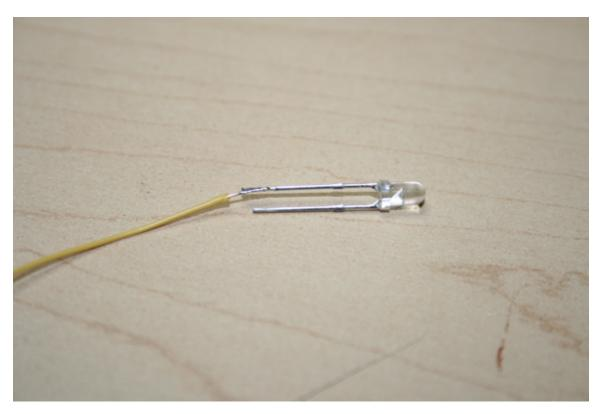
If using a DBU, connect a wire from the **long** leg of the supplied IR led to the *innermost* pin of the connection point labeled IRLED. This wire should be immediately next to the location R1
