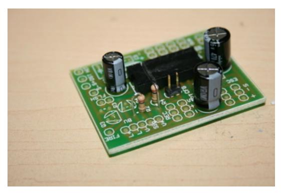
Solder in two 200k ohm resistors (red, black, yellow) at R2 and R4, a 470uF capacitor at C4, and a 1uF capacitor at C1. Make sure the capacitors match the polarity on the silkscreen.
