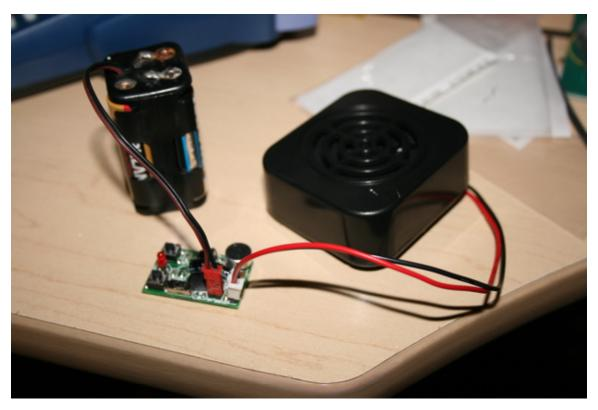
Connect a 5-6V battery (a JST plug fits nicely) using the marked polarity and record the appropriate sounds. The instructions are available at http://www.electronics123.net/amazon/datasheet/A96020.pdf. (basically flip the switch to rec and hold down the appropriate button, release to finish, move switch to play and hit button to demo)
