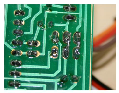
**IMPORTANT**: There is a minor PCB error on version1 boards. The "+" and "-" traces between the "OPT" and "REC" need to be joined. **Boards** marked "v2" do not need this fix.
