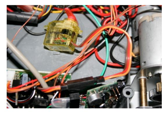
You may optionally connect a micro servo the connector soldered to "REC" earlier. This servo **must** be a micro servo, or the power requirements may cause the DBC to reset or reboot sporadically. With some micro servos, a heatsink may still be required on the voltage regulator for reliable operation.
