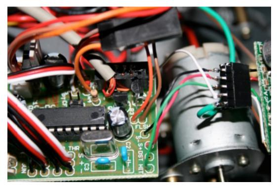
Connect a red wire to the **long** leg of the white LED and connect this wire to the *innermost* pin of the socket labeled "FLSH". Connect a black or brown wire to the **short** leg of the white LED and connect it to the *outermost* pin of the socket.
