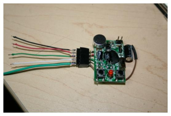
Connect the wires to the optional header and pin connectors. This makes it easier to pull the sound chip off for future recordings.
