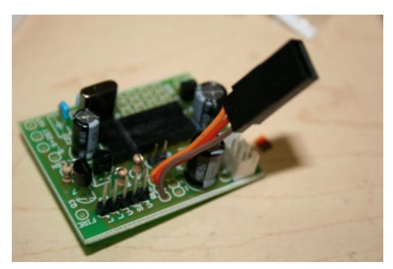
Cut the five servo extensions, leaving enough wire on the "plug" side to reach from the DBC to your receiver location.
