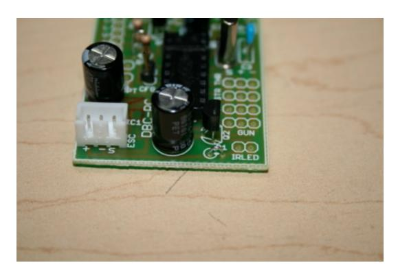
Install the socket at "ESC". Note the orientation as shown.
