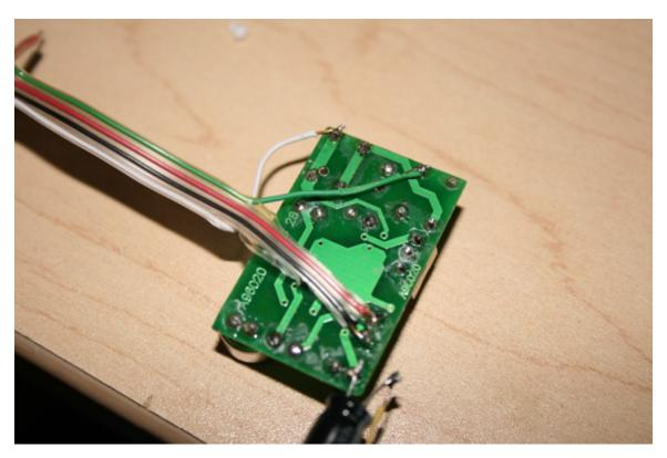
Solder a red wire to the underside of the 6v pin, and a black wire to the underside of the ground pin. Solder two wires to these locations under the buttons. Keep track of which wire is connected to which button.
