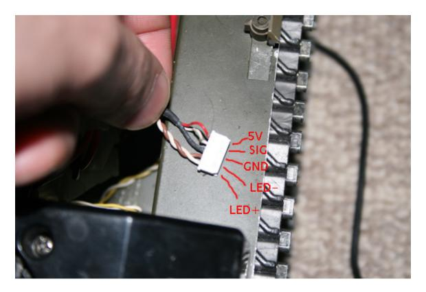
If fitting a TBU, use this pinout to connect to the DBC-RC2HL board. You will need to cut the connector off though.
