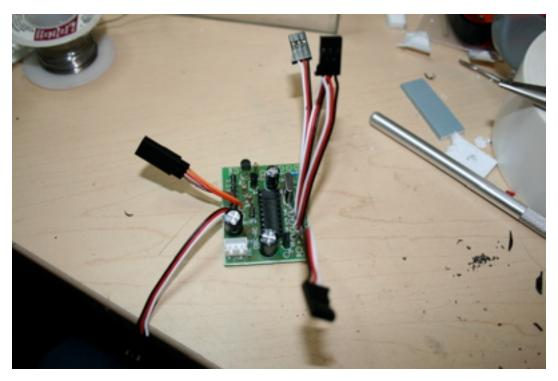
Install the five servo plugs into locations "THR, STR, TUR, GUN" and optionally "OPT" (for five channel radios). Wire colors may differ, so note the polarity (Red=+, Black/Brown=-, Orange/White=s).
