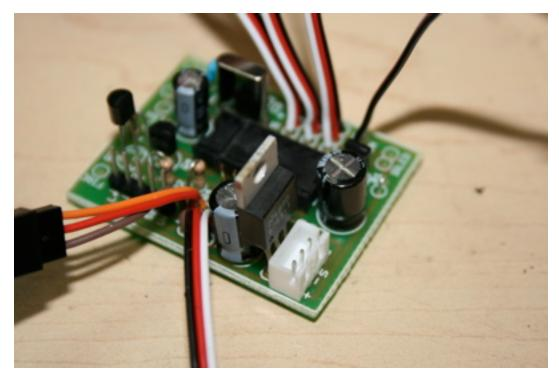
Install the voltage regulator at location IC1. You may want to locate it closer to the board than shown to make the DBC easier to mount.
