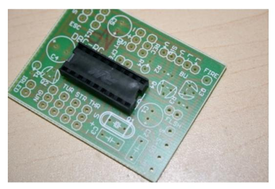
Solder the 18 pin socket onto the PCB. Make sure you line up the full notch with the small "D" shape marker on the silkscreen.
