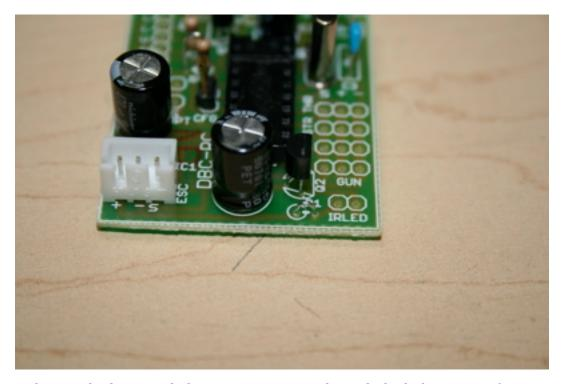
If using the supplied DBU IR led, connect a jumper through the holes at R1. If using another IR LED, you may need to use a resistor between 10 and 68 ohms to equalize the range and prevent led burnout.
