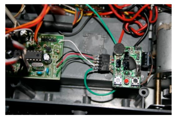
Connect the Red (+) wire to "S+" and the Black (-) wire to "S-". Connect the sound trigger wires to the desired outputs "Hit", "Dst" (destroyed), or "Fire". In this picture, "Hit" and "Fire" are used.
